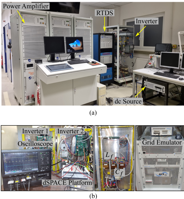
Fig. 23. (a) Picture of the experimental setup 1: single converter connected to the grid. (b) Picture of the experimental setup 2: two converters operating in parallel to the grid.
