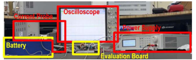
Fig. 31. Measurement setup of the charger system with proposed MBD BLS.
