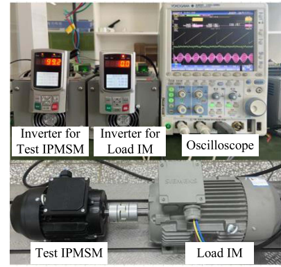
Fig. 12. 2.2-kW IPMSM experimental platform.
