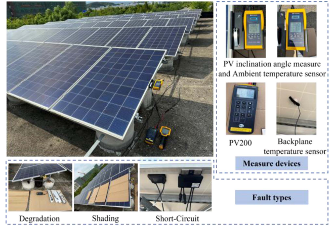
Fig. 12. Experiment platform and fault simulation.
