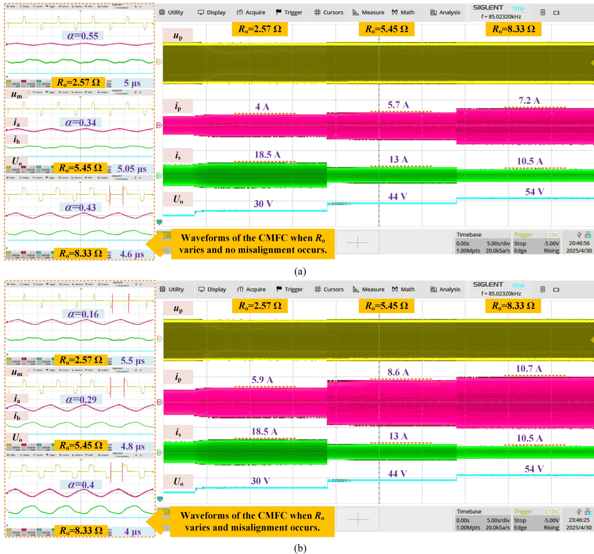
Fig. 21. Experimental waveforms during the dynamic charging process. (a) \Delta x = 0 and \Delta y = 0 . (b) \Delta x = 37.7\% and \Delta y = 0 .
