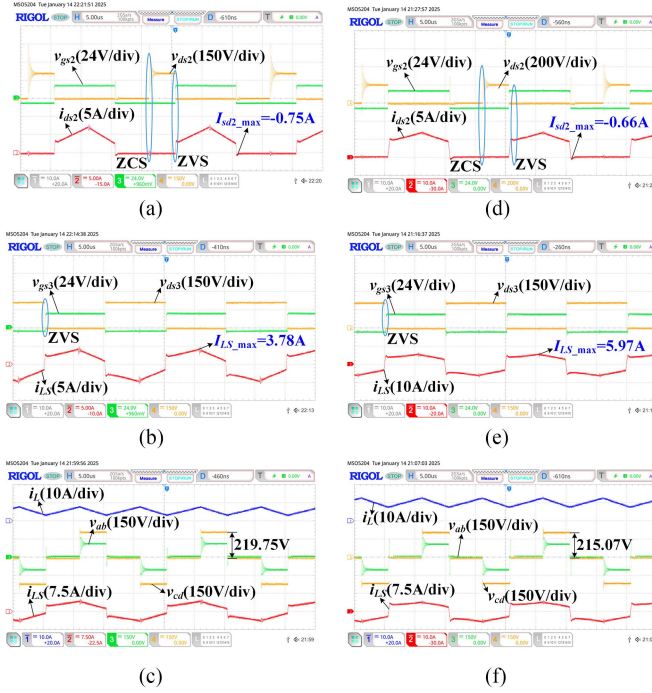
Fig. 15. Experimental waveforms of the proposed CCS strategy under Case 2. (a)–(c) Half-load. (d)–(f) Full-load.
