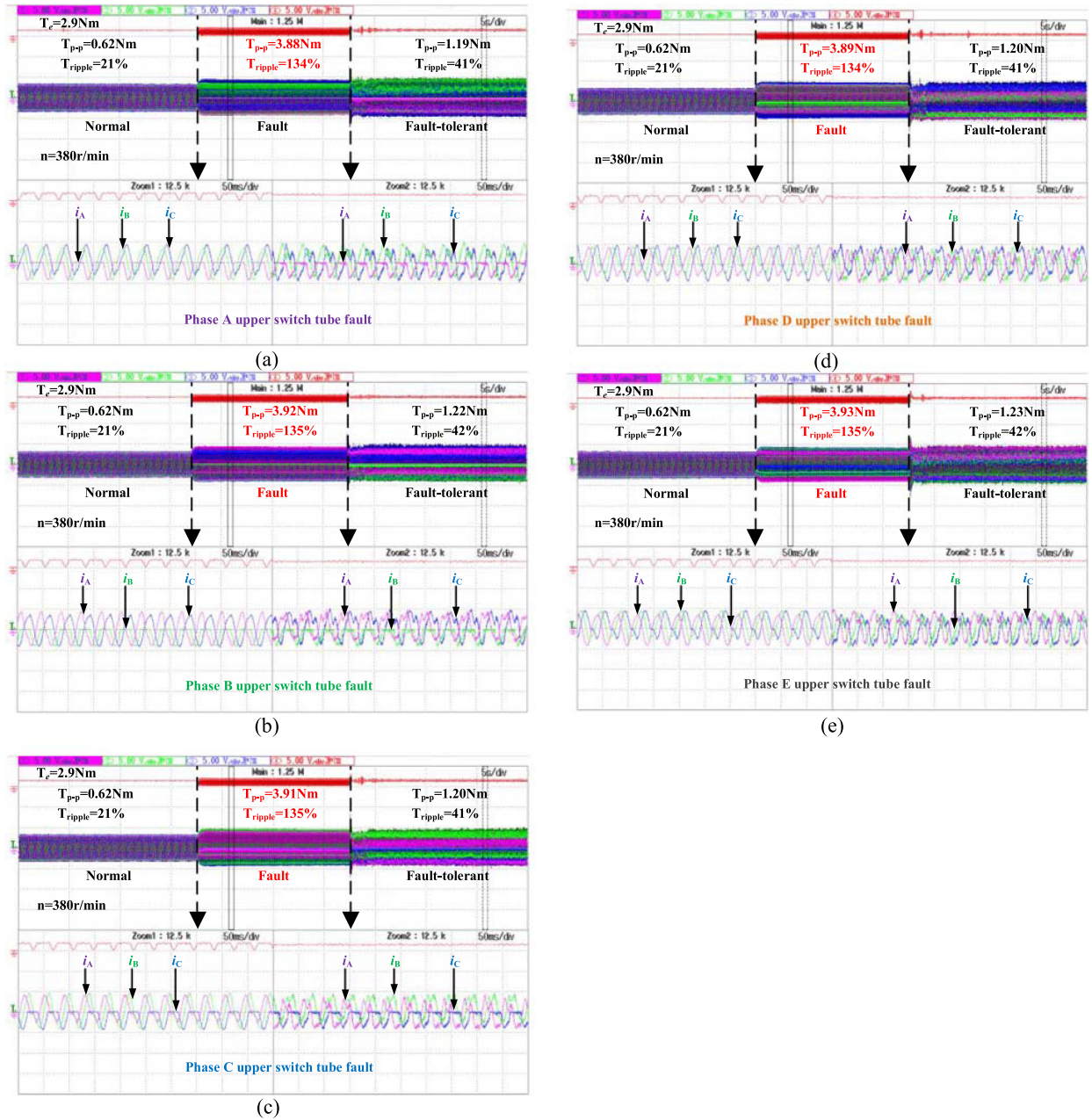
Fig. 35. Torque and currents waveforms from normal operation to fault and fault-tolerant operation. (a) Phase A upper switch tube fault. (b) Phase B upper switch tube fault. (c) Phase C upper switch tube fault. (d) Phase D upper switch tube fault. (e) Phase E upper switch tube fault. T_e is scaled to 10 Nm/div, phase currents are scaled to 5 A/div.
