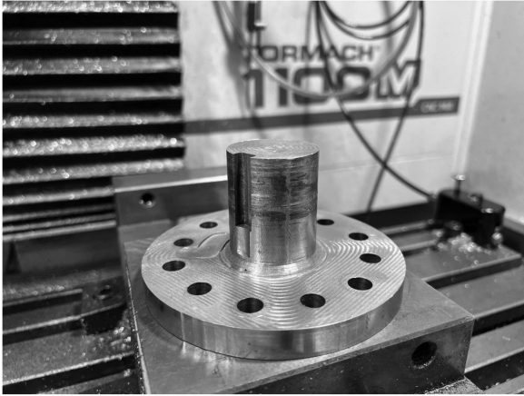
Fig. 18. Custom shaft coupler machined at NCREPT using the Tormach 1100 M CNC.
