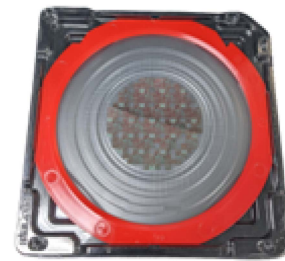
Fig. 2. 4H-SiC wafer having the planar CMOS gate drivers fabricated.
