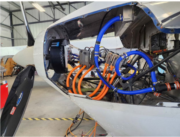
Fig. 24. Final integration of SiC inverter into test airframe.
