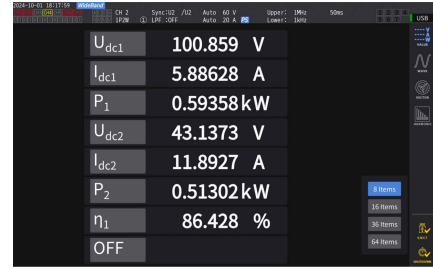
Fig. 24. System electrical parameters in a perfect-alignment.
