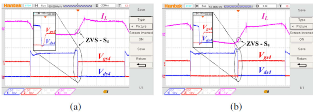
Fig. 18. Steady state waveforms of HFT current i_L , V_{ds} and V_{gs} with the proposed optimization strategy for (a) k = 0.9 and (b) k = 1.1 .
