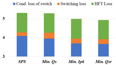
Fig. 17. Power loss components (in Watts) for output power of 80 W.
