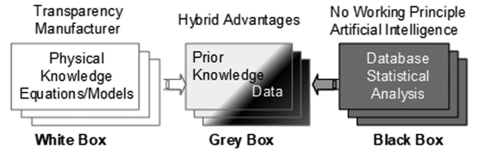
Fig. 6. Schematic diagram of basic principles of white box, grey box, and black box for insulation systems.
