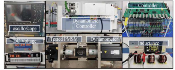
Fig. 10. Experimental system of permanent magnet synchronous motor.
