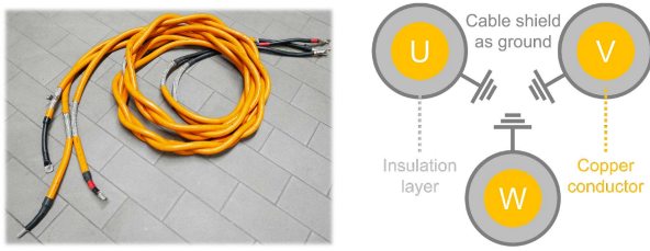
Fig. 4. Modeled cable set.
