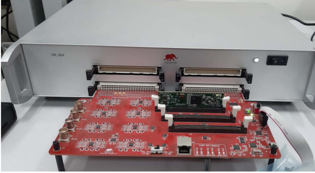
Fig. 6. Typhoon HIL-604, \mu grid DSP interface board, and TMS320F28335 microcontroller used in the HIL verification.
