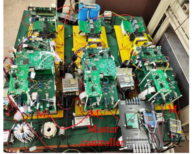
Fig. 15. Photograph of the three-module SST prototype.
