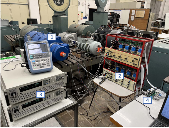
Fig. 15. Photograph of the experimental setup: 1—Ward-Leonard machine set with 12-kW induction and 8.8-kW DC machine, 2—SiC inverter, 3—bidirectional dc supplies, 4—DSP control board.
