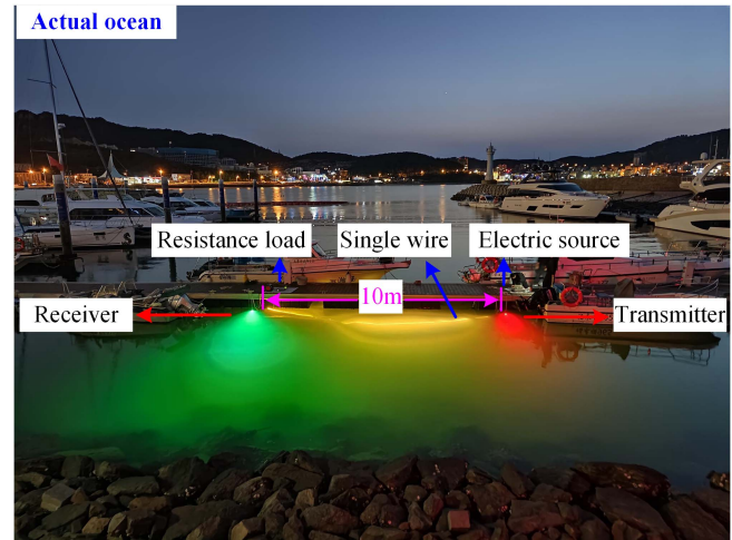
Fig. 25. Prototype of the SCPT system with single wire in the actual ocean.
