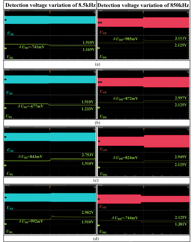
Fig. 24. Detection voltage signal variations of different FOs intrusion. (a) 40 \times 40 mm copper intrude. (b) 40 \times 40 mm aluminium intrude. (c) 40 \times 40 mm iron intrude.
