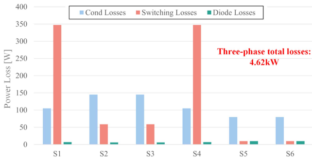
Fig. 29. Loss breakdown of switches in one phase leg under the half-load condition.
