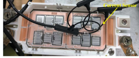
Fig. 6. Experimental test bench for evaluating collector current.
