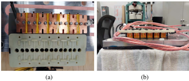
Fig. 13. Compensation capacitor bank used in the demonstrators. (a) View of the disassembled compression plate, bus bars, and capacitors. (b) Side view of the assembled capacitor bank mounted on the Gen. 1 coil assembly.
