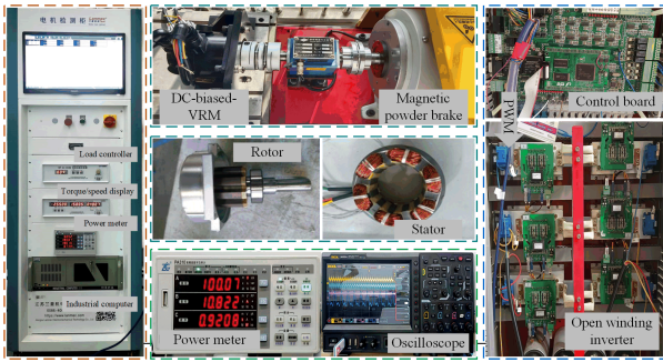
Fig. 8. Experimental equipment diagram.
