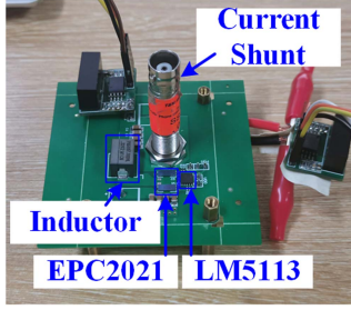
Fig. 15. Hardware prototype of the synchronous buck converter.
