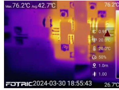
Fig. 14. Thermal distribution of the prototype with forced air cooling.
