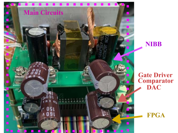
Fig. 18. Photograph of main circuits.
