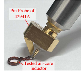
Fig. 38. Test setup of the air-core inductors.
