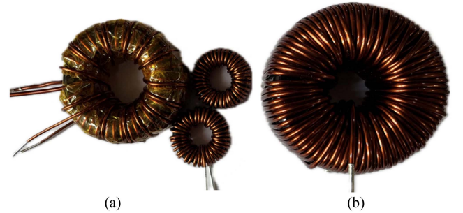
Fig. 12. Inductors in the (a) improved circuit and (b) conventional circuit.
