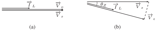
Fig. 9. FHA phasor diagrams of the LCC-CF for ZVS angle considerations. (a) Mode AB. (b) Mode B.
