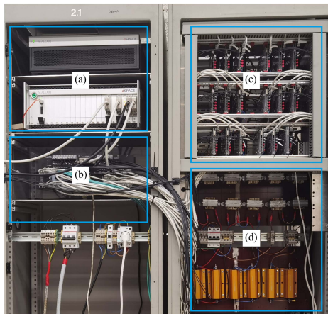
Fig. 5. Setup of the testbench. (a) dSPACE SCALEXIO real-time system. (b) Interface. (c) Three phase MMC. (d) RL load.
