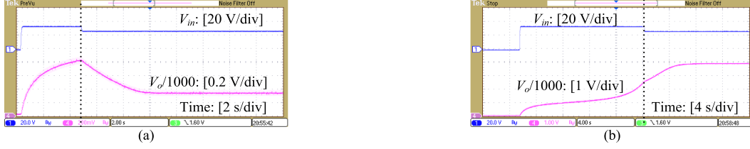
Fig. 18. Open-loop dynamic response of V_o to different step change of V_{in} of #2 prototype with compensation parameters in Table VIII. (a) V_{in} is set from 35 V to 28 V when V_o=0.8 kV. (b) V_{in} is set from 35 to 28 V when V_o=2.56 kV.
