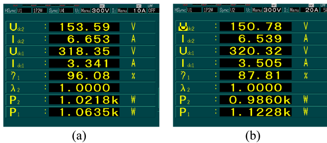
Fig. 14. Power meter. (a) Well aligned. (b) 120-mm vertical misalignment.
