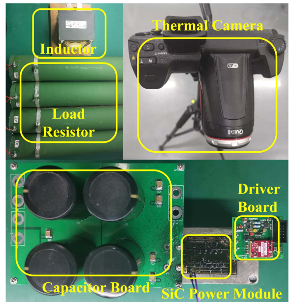
Fig. 18. Experimental test rig for evaluating the accuracy of the proposed cosimulation method.
