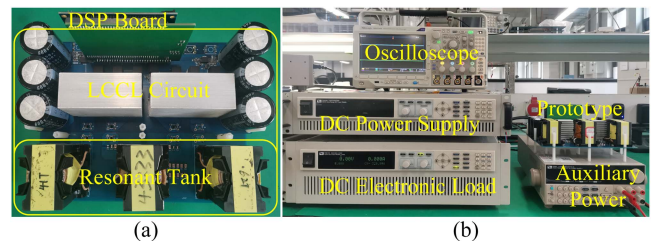
Fig. 20. Experimental setup. (a) LCCL prototype. (b) Experimental test platform.
