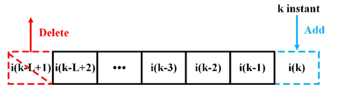
Fig. 4. Operation rule of the sliding windows.
