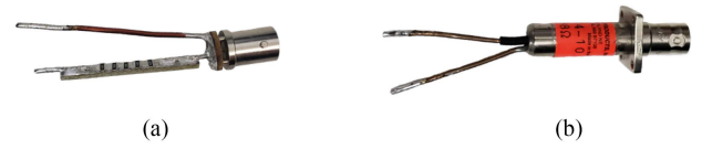
Fig. 5. Probes used to measure. (a) Voltage. (b) Current.
