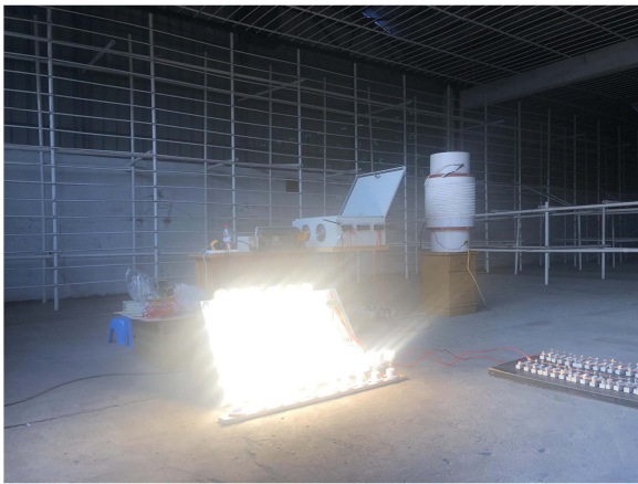
Fig. 25. Power of 5 kW is transmitted at a transmission distance of 5 km.
