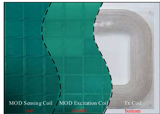
Fig. 23. MOD coil sets structure diagram.
