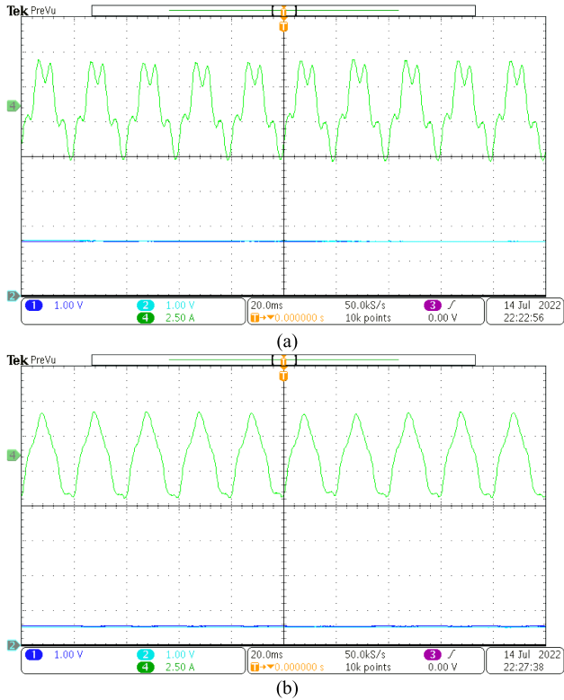
Fig. 21. Experimental waveforms of the grid current and the SACS current amplitude in GC mode (a) without SACS current limiting, and (b) with SACS current limiting; CH1, I_{os1} , 0.4 A/div; CH2, I_{os2} , 0.4 A/div; CH4, i_{ga} , 2.5 A/div.
