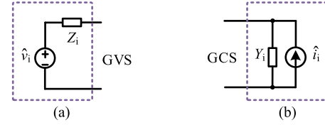
Fig. 5. Equivalent circuits: (a) Thevenin equivalent circuit for GVS and (b) Norton equivalent circuit for GCS.
