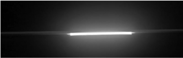
Fig. 16. Photo of DBD phenomenon during work.
