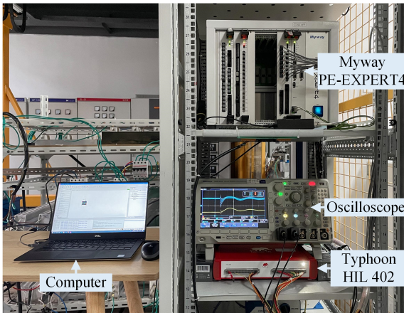
Fig. 10. Control hardware-in-loop experimental platform.
