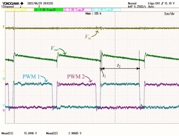
Fig. 20. Waveforms of V_{in} , V_{out} , PWM 1 and PWM 2 at d = 0.45 and f_s = 100 kHz.
