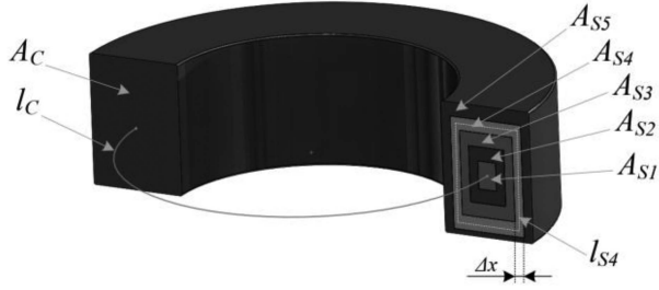
Fig. 17. Magnetic core conceptually divided into five concentric shells.
