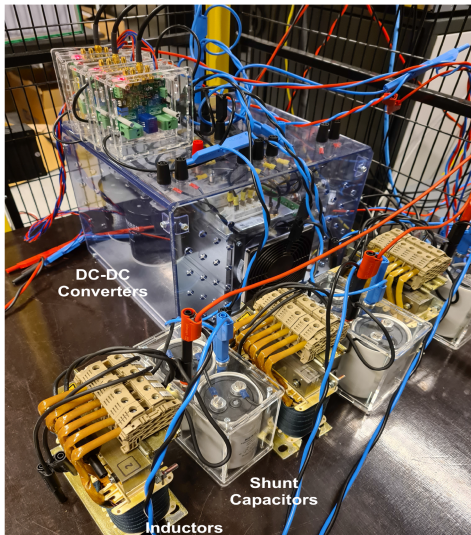
Fig. 6. Experimental setup of a dc microgrid consisting of n = 3 DG units.
