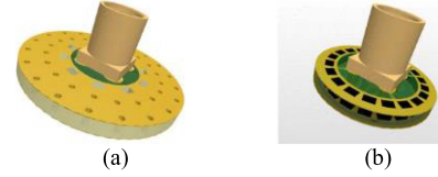
Fig. 3. Two proposed surface mount coaxial shunt resistor PCB designs in [18].
