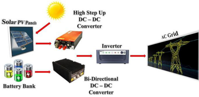
Fig. 1. Block diagram of a grid-connected renewable energy system.
