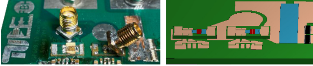
Fig. 14. PCB HB setup modified for VNA measurement (left) and the corresponding 3-D model employed in FEM field simulation (right).
