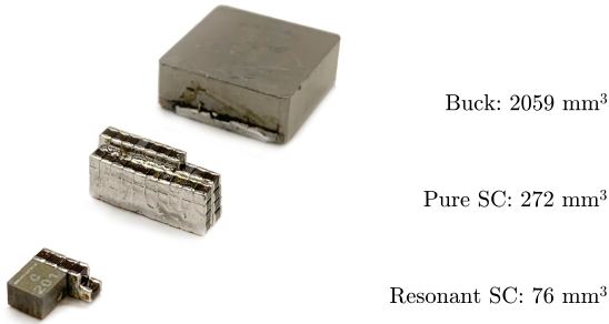
Fig. 10. Required passive component volume to achieve the efficiency performance shown in Fig. 9.
