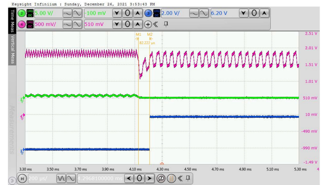
Fig. 19. Waveforms of input current (500 mA/div), inductor current of phase-1 (5 A/div), and indicator under OCF in phase-1; time scale = 200 \mu s/div.
