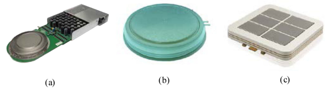
Fig. 1. Photographs of main high-power semiconductors for the MMC-HVdc system. (a) IGCT. (b) Press-pack IEGT. (c) StakPak IGBT.
